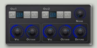
Select the oscillators waveform (sine, saw, triangle or square) and adjust the volume and octave for each oscillator. Detune the second oscillator frequency with DETUNE knob. With NOISE knob white noise can be added to the sound texture.
